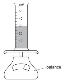
Some more of the liquid is added until the liquid level reaches the 50 cm<sup>3</sup> mark.
